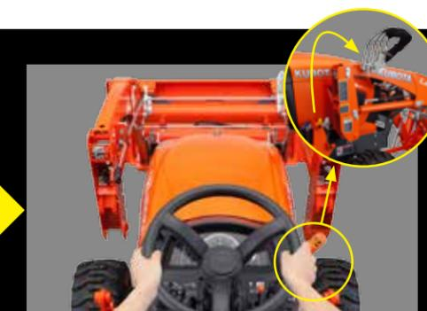
**Step 4:** Pull one lever to quickly and easily detach the hydraulic lines as a unit and store the coupler on the loader boom.
