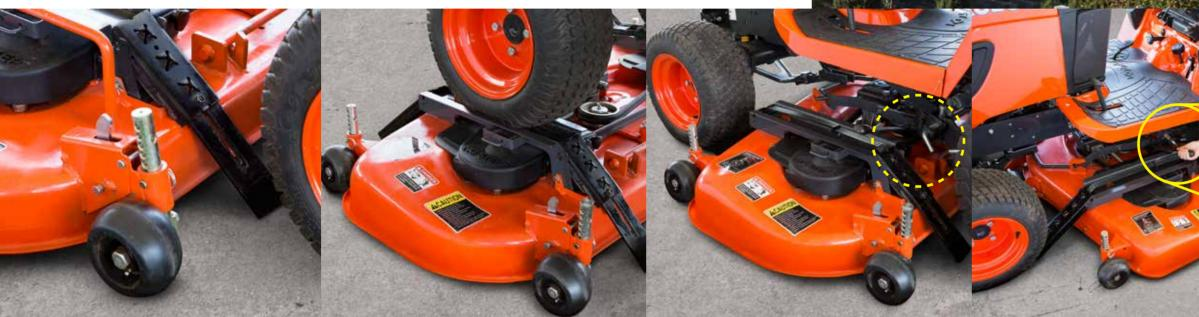
**Step 1:** Slide out the ramps and release the gauge wheels. Step 2: Drive over the deck.
