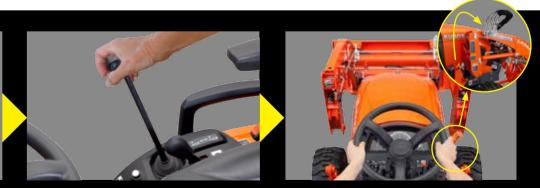
Step 3: Use the loader lever to remove the loader frame from the mast. Turn off the engine and move the loader joystick lever to relieve the hydraulic pressure.
