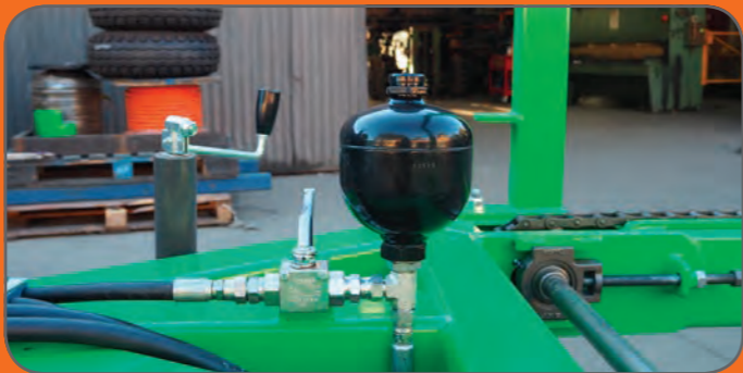
Soft ride hydraulic suspension accumulator
