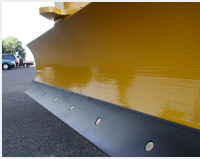
Manganese hardened steel cutting edge
