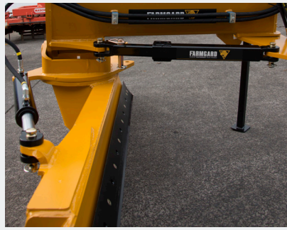
85% of total weight on cutting edge
