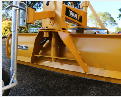
85% of total weight on cutting edge
