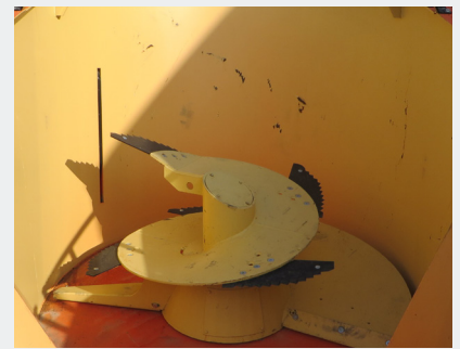
Vertical auger with tungsten knives
