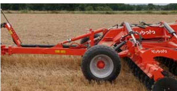
On trailed models additional gauge wheels of 340/55x16 (option) can be mounted in front of the discs to ensure better machine stability and a constant depth control during operation. The working depth can be easily adjusted by spacers at the depth cylinders as with the rollers.
