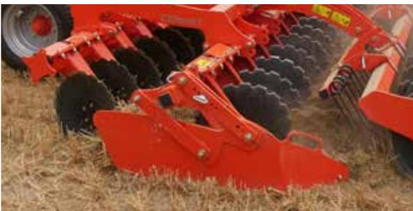
The adjustable lateral side deflectors on the right and left-hand side control the soil flow to provide a perfect level finish. All discs are working at the same depth, even the outer ones. The lateral deflectors are parallelogram mounted which allows them to follow the ground contours and control the soil flow at the same time.
