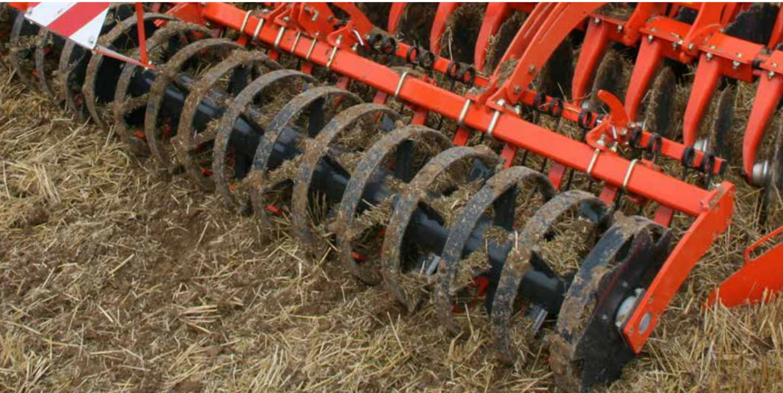
Consolidation is an elementary action of arable farming. Reducing large open pores and aggregate size allows for improved seed-to-soil contact and keeping the water necessary for the next crop germination. The right choice of the right roller depends on the soil type and conditions. Also, lifting capacity of the tractor needs to be considered. Therefore, Kubota offers a wide range of maintenance-free rollers to finalise the levelling and re-consolidation of the soil.
