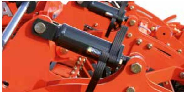
The working depth can easily be adjusted by pivoting spacers, no matter if it is manually (only on mounted models) or hydraulically.
