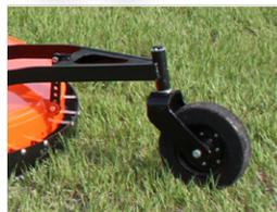
The laminated tailwheel is long lasting in rough conditions and 1-1/2" heavy-duty spindle protects the assembly.
