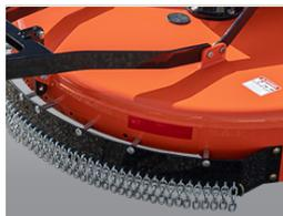
Optional shields are available for the front and rear to protect against flying debris.
